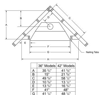
68 <sup>1</sup>/<sub>2</sub>" Figure 5 - Framing Clearances for Corner Installation
